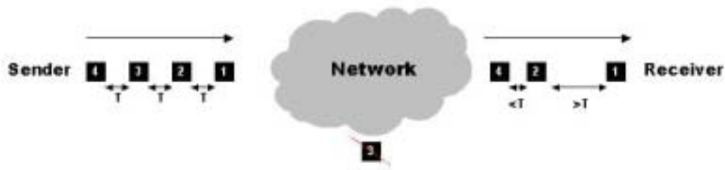
Figure 2: Illustration of packets traversing the network. Packet 3 was dropped, whilst the other packets arrived with variable delay.
